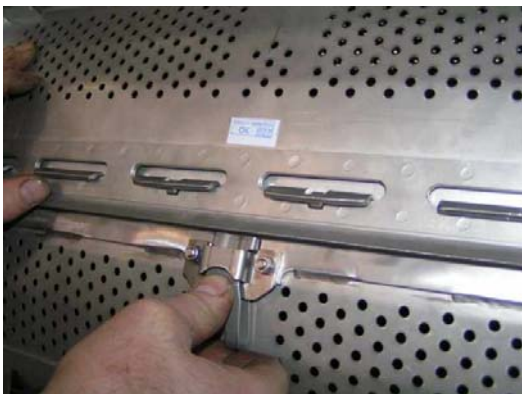
First phase of opening the door. Press safety pin spring.
