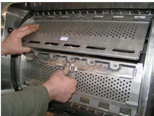
Using both hands force push both door parts inside until the latches on one door part are released from the openings on the other door part.
